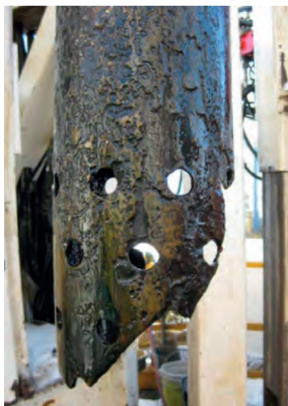
Fig. 3. Heavy corrosion of liner pipe in the KJ-39 well (source: deliverable D4.3 from GeoWell project, Þorbjörnsson 2016)
