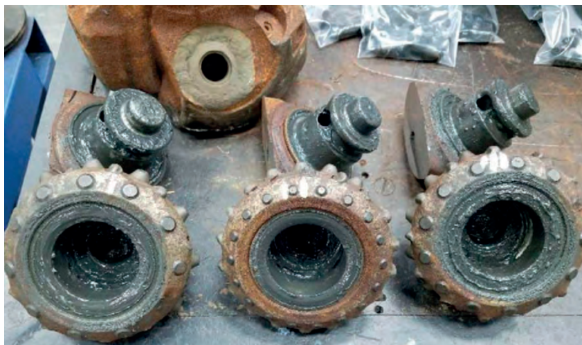
Fig. 1. Cones and bearing from high-temperature tri-cone roller cone drill bits used during drilling of the IDDP-2 well in the Reykjanes geothermal field in Iceland (Stefánsson et al. 2018)
