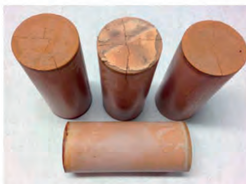
Thermalock after 7 day exposure to 450°C
