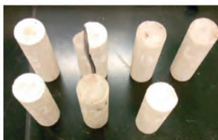
Geoterm™ / 70% silica after 7 day exposure to 450°C
